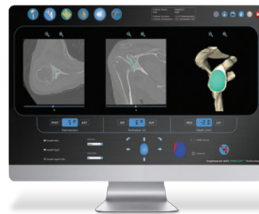
Figure 2. Main window of BLUEPRINT™ 3D Planning Software for selecting the suitable position of the glenoid implant in accordance to the version, the inclination, the reaming depth and the seating.
